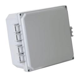
Integra Premium series enclosure, NEMA 1/2/3/3R/3S/4/4X/12/13, 8 x 8 x 4in (HxWxD), wall mount, polycarbonate, light gray, gloss finish, single-door, glass-filled nylon quick-release latch, padlock hasp and staple.
