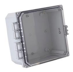
Integra Premium series enclosure, NEMA 1/2/3/3R/3S/4/4X/12/13, 8 x 8 x 4in (HxWxD), wall mount, polycarbonate, light gray, gloss finish, clear polycarbonate singledoor, glass-filled nylon quick-release latch, padlock hasp and staple.
