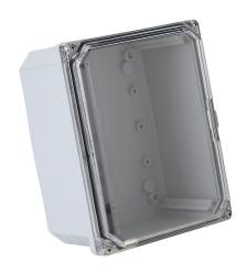
Integra Premium series enclosure, NEMA 1/2/3/3R/3S/4/4X/6/6P/12/13, 8 x 6 x 4in (HxWxD), wall mount, polycarbonate, light gray, gloss finish, clear polycarbonate screw cover.
