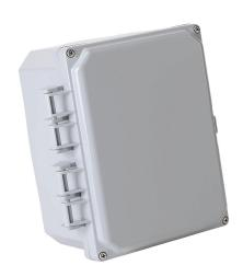
Integra Premium series enclosure, NEMA 1/2/3/3R/3S/4/4X/6/6P/12/13, 8 x 6 x 4in (HxWxD), wall mount, polycarbonate, light gray, gloss finish, hinged screw cover.
