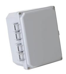
Integra Premium series enclosure, NEMA 1/2/3/3R/3S/4/4X/6/6P/12/13, 8 x 6 x 4in (HxWxD), wall mount, polycarbonate, light gray, gloss finish, hinged screw cover.
