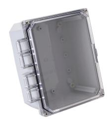
Integra Premium series enclosure, NEMA 1/2/3/3R/3S/4/4X/6/6P/12/13, 8 x 6 x 4in (HxWxD), wall mount, polycarbonate, light gray, gloss finish, clear polycarbonate hinged screw cover.
