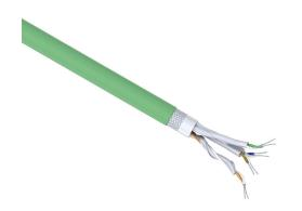
Helukabel HELUKAT flexible Cat6a industrial Ethernet cable, individual and overall shielded, 4 twisted pairs, 24 AWG, 7-stranded, tinned copper, foam polyethylene conductor insulation material, PVC jacket, green, cut to length.
