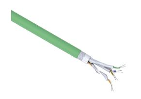
Helukabel HELUKAT flexible Cat6a industrial Ethernet cable, individual and overall shielded, 4 twisted pairs, 24 AWG, 7-stranded, tinned copper, foam polyethylene conductor insulation material, PUR jacket, green, cut to length.
