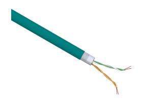
Helukabel HELUKAT flexible Cat5e industrial Ethernet cable, overall shielded, 2 twisted pairs, 26 AWG, 7-stranded, bare copper, foam polyethylene conductor insulation material, PUR jacket, blue, cut to length.
