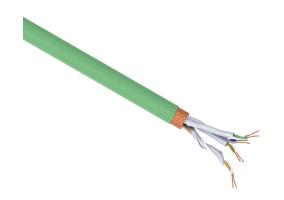
Helukabel HELUKAT Cat7a industrial Ethernet cable, individual and overall shielded, 4 twisted pairs, 23 AWG, solid, bare copper, foam polyethylene conductor insulation material, polyurethane (PUR) jacket, green, cut to length.
