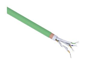
Helukabel HELUKAT flexible Cat7 industrial Ethernet cable, individual and overall shielded, 4 twisted pairs, 24 AWG, 7-stranded, tinned copper, foam polyethylene conductor insulation material, PUR jacket, green, cut to length.
