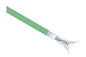
Helukabel HELUKAT flexible Cat6a industrial Ethernet cable, overall shielded, 4 twisted pairs, 26 AWG, 7-stranded, tinned copper, foam polyethylene conductor insulation material, PUR jacket, green, cut to length.
