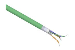
Helukabel HELUKAT continuous flexing Cat6 industrial Ethernet cable, overall shielded, 4 twisted pairs, 26 AWG, 19-stranded, tinned copper, polypropylene conductor insulation material, PUR jacket, green, cut to length.
