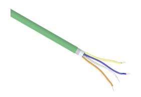
Helukabel HELUKAT continuous flexing Profinet Type C cable, overall shielded, 1 star quad, 22 AWG, 19-stranded, tinned copper, polyethylene conductor insulation material, PUR jacket, green, cut to length.
