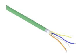
Helukabel HELUKAT flexible Profinet Type B cable, overall shielded, 1 star quad, 22 AWG, 7-stranded, tinned copper, FRNC conductor insulation material, FRNC jacket, green, cut to length.
