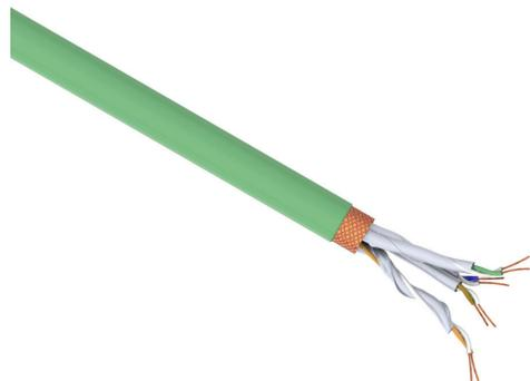
Helukabel HELUKAT flexible Cat7 industrial Ethernet cable, individual and overall shielded, 4 twisted pairs, 26 AWG, 7-stranded, bare copper, foam polyethylene conductor insulation material, PUR jacket, green, cut to length.
