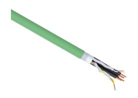
Helukabel HELUKAT flexible Profinet Type B cable, individual and overall shielded, (2) shielded twisted pairs, (4) unshielded conductors, 22 AWG and 16 AWG, 7-stranded, bare copper, polyethylene conductor insulation material, FRNC jacket, green, cut to length.
