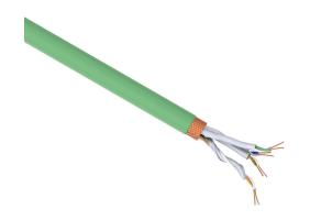
Helukabel HELUKAT Cat7e industrial Ethernet cable, individual and overall shielded, 4 twisted pairs, 23 AWG, solid, bare copper, foam polyethylene conductor insulation material, polyurethane (PUR) jacket, green, cut to length.
