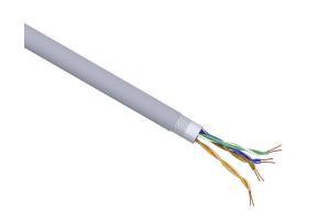
Helukabel HELUKAT flexible Cat5e industrial Ethernet cable, overall shielded, 4 twisted pairs, 26 AWG, 7-stranded, bare copper, polyolefin conductor insulation material, PUR jacket, gray, cut to length.
