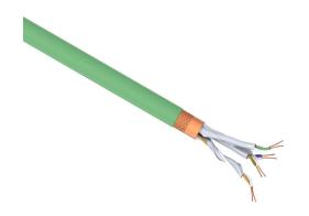
Helukabel HELUKAT continuous flexing Cat5 industrial Ethernet cable, individual and overall shielded, 4 twisted pairs, 26 AWG, 19-stranded, bare copper, polypropylene conductor insulation material, PUR jacket, green, cut to length.
