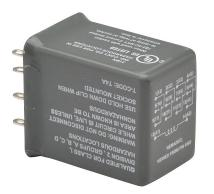
AutomationDirect ice cube control relay, socket mount, hermetically sealed, 24 VDC coil voltage, 4PDT, (4) N.O., (4) N.C., 5A contact rating, 14-pin. Requires 782-4C-SKT mounting socket. Hazardous location certified.
