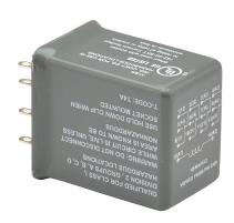
AutomationDirect ice cube control relay, socket mount, hermetically sealed, 24 VAC coil voltage, 4PDT, (4) N.O., (4) N.C., 5A contact rating, 14-pin. Requires 782-4C-SKT mounting socket. Hazardous location certified.
