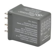
AutomationDirect ice cube control relay, socket mount, hermetically sealed, 240 VAC coil voltage, 4PDT, (4) N.O., (4) N.C., 5A contact rating, 14-pin, LED indicator(s). Requires 782-4C-SKT mounting socket. Hazardous location certified.
