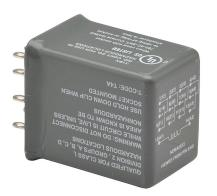
AutomationDirect ice cube control relay, socket mount, hermetically sealed, 12 VDC coil voltage, 4PDT, (4) N.O., (4) N.C., 5A contact rating, 14-pin. Requires 782-4C-SKT mounting socket. Hazardous location certified.
