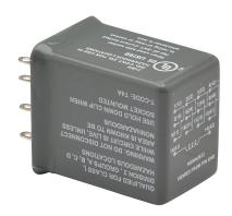
AutomationDirect ice cube control relay, socket mount, hermetically sealed, 12 VAC coil voltage, 4PDT, (4) N.O., (4) N.C., 5A contact rating, 14-pin, LED indicator(s). Requires 782-4C-SKT mounting socket. Hazardous location certified.
