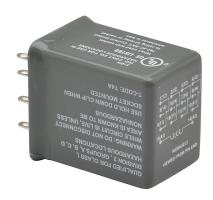
AutomationDirect ice cube control relay, socket mount, hermetically sealed, 12 VAC coil voltage, 4PDT, (4) N.O., (4) N.C., 5A contact rating, 14-pin. Requires 782-4C-SKT mounting socket. Hazardous location certified.
