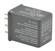
AutomationDirect ice cube control relay, socket mount, hermetically sealed, 120 VAC coil voltage, 4PDT, (4) N.O., (4) N.C., 5A contact rating, 14-pin. Requires 782-4C-SKT mounting socket. Hazardous location certified.
