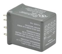
AutomationDirect ice cube control relay, socket mount, hermetically sealed, 24 VAC coil voltage, 4PDT, (4) N.O., (4) N.C., 3A contact rating, 14-pin. Requires 782-4C-SKT mounting socket. Hazardous location certified.
