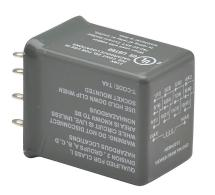
AutomationDirect ice cube control relay, socket mount, hermetically sealed, 240 VAC coil voltage, 4PDT, (4) N.O., (4) N.C., 3A contact rating, 14-pin. Requires 782-4C-SKT mounting socket. Hazardous location certified.
