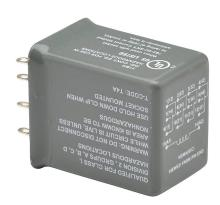
AutomationDirect ice cube control relay, socket mount, hermetically sealed, 12 VDC coil voltage, 4PDT, (4) N.O., (4) N.C., 3A contact rating, 14-pin. Requires 782-4C-SKT mounting socket. Hazardous location certified.
