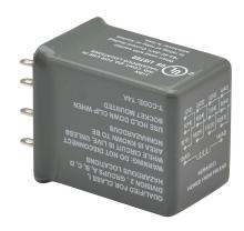
AutomationDirect ice cube control relay, socket mount, hermetically sealed, 12 VAC coil voltage, 4PDT, (4) N.O., (4) N.C., 3A contact rating, 14-pin. Requires 782-4C-SKT mounting socket. Hazardous location certified.
