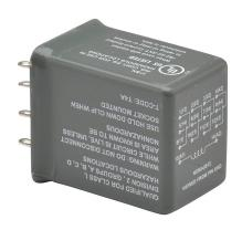
AutomationDirect ice cube control relay, socket mount, hermetically sealed, 120 VAC coil voltage, 4PDT, (4) N.O., (4) N.C., 3A contact rating, 14-pin, LED indicator(s). Requires 782-4C-SKT mounting socket. Hazardous location certified.
