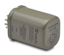
AutomationDirect octal control relay, socket mount, hermetically sealed, 24 VDC coil voltage, 3PDT, (3) N.O., (3) N.C., 12A contact rating, 11-pin. Requires 750-3C-SKT mounting socket. Hazardous location certified.
