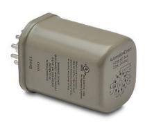
AutomationDirect octal control relay, socket mount, hermetically sealed, 24 VAC coil voltage, 3PDT, (3) N.O., (3) N.C., 12A contact rating, 11-pin. Requires 750-3C-SKT mounting socket. Hazardous location certified.
