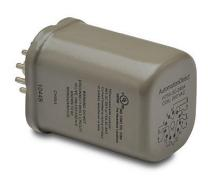
AutomationDirect octal control relay, socket mount, hermetically sealed, 240 VAC coil voltage, 3PDT, (3) N.O., (3) N.C., 12A contact rating, 11-pin, LED indicator(s). Requires 750-3C-SKT mounting socket. Hazardous location certified.
