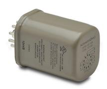
AutomationDirect octal control relay, socket mount, hermetically sealed, 12 VAC coil voltage, 3PDT, (3) N.O., (3) N.C., 12A contact rating, 11-pin. Requires 750-3C-SKT mounting socket. Hazardous location certified.
