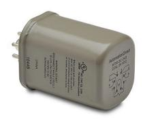
AutomationDirect octal control relay, socket mount, hermetically sealed, 24 VDC coil voltage, DPDT, (2) N.O., (2) N.C., 12A contact rating, 8-pin. Requires 750-2C-SKT mounting socket. Hazardous location certified.
