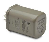
AutomationDirect octal control relay, socket mount, hermetically sealed, 24 VAC coil voltage, DPDT, (2) N.O., (2) N.C., 12A contact rating, 8-pin. Requires 750-2C-SKT mounting socket. Hazardous location certified.
