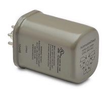
AutomationDirect octal control relay, socket mount, hermetically sealed, 240 VAC coil voltage, DPDT, (2) N.O., (2) N.C., 12A contact rating, 8-pin. Requires 750-2C-SKT mounting socket. Hazardous location certified.
