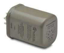
AutomationDirect octal control relay, socket mount, hermetically sealed, 12 VDC coil voltage, DPDT, (2) N.O., (2) N.C., 12A contact rating, 8-pin. Requires 750-2C-SKT mounting socket. Hazardous location certified.
