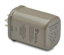
AutomationDirect octal control relay, socket mount, hermetically sealed, 120 VAC coil voltage, DPDT, (2) N.O., (2) N.C., 12A contact rating, 8-pin. Requires 750-2C-SKT mounting socket. Hazardous location certified.
