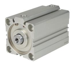
NITRA pneumatic cylinder, compact extruded, 63mm bore, 20mm rod diameter, 75mm stroke, double acting, magnetic piston, tapped end caps mount.
