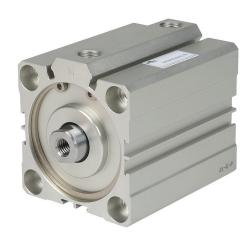
NITRA pneumatic cylinder, compact extruded, 63mm bore, 20mm rod diameter, 50mm stroke, double acting, magnetic piston, tapped end caps mount.
