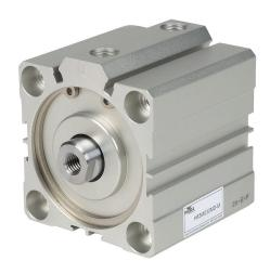
NITRA pneumatic cylinder, compact extruded, 63mm bore, 20mm rod diameter, 30mm stroke, double acting, magnetic piston, tapped end caps mount.
