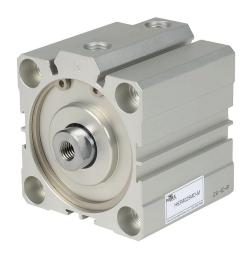
NITRA pneumatic cylinder, compact extruded, 63mm bore, 20mm rod diameter, 25mm stroke, double acting, magnetic piston, tapped end caps mount.
