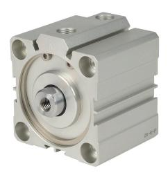
NITRA pneumatic cylinder, compact extruded, 63mm bore, 20mm rod diameter, 20mm stroke, double acting, magnetic piston, tapped end caps mount.
