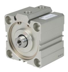
NITRA pneumatic cylinder, compact extruded, 63mm bore, 20mm rod diameter, 15mm stroke, double acting, magnetic piston, tapped end caps mount.
