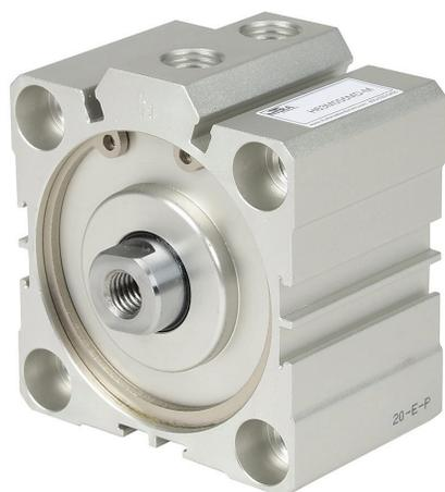
NITRA pneumatic cylinder, compact extruded, 63mm bore, 20mm rod diameter, 5mm stroke, double acting, magnetic piston, tapped end caps mount.
