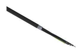
Helukabel TOPFLEX 600 VFD cable, shielded, 4 conductors (includes ground), 2 AWG, tinned copper, XLPE conductor insulation material, black with white numbers and green/yellow ground, PVC jacket, black, cut to length.
