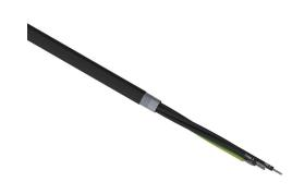
Helukabel TOPFLEX 600 VFD cable, shielded, 4 conductors (includes ground), 4 AWG, tinned copper, XLPE conductor insulation material, black with white numbers and green/yellow ground, PVC jacket, black, cut to length.
