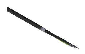
Helukabel TOPFLEX 600 VFD cable, shielded, 4 conductors (includes ground), 6 AWG, tinned copper, XLPE conductor insulation material, black with white numbers and green/yellow ground, PVC jacket, black, cut to length.
