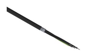
Helukabel TOPFLEX 600 VFD cable, shielded, 4 conductors (includes ground), 8 AWG, tinned copper, XLPE conductor insulation material, black with white numbers and green/yellow ground, PVC jacket, black, cut to length.
